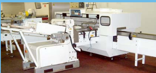
Ibonhart bagging and slicing line, fully automatic feed system complete with bagger, slicer and conveying.
