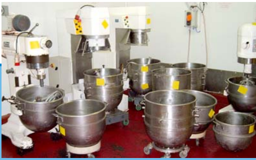
Numerous spiral, paddle and high speed mixers of various capacity and speeds all with stainless steel bowls and tooling.
