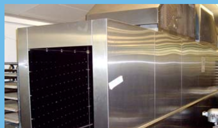
Acrivan six rack ambient stainless steel prover manufactured 2003.
