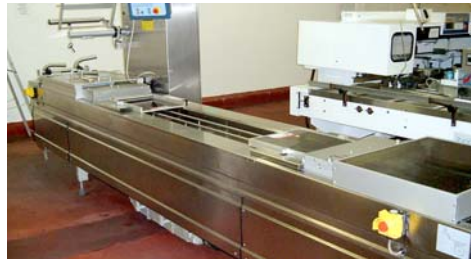
Multivac R230 Yr 2002 thermo-former with numerous tooling, plc menu control fully automatic. Also available Meca 320 gas flush tray sealer & Multivac TS355 tray sealers.
