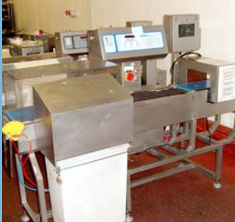
Numerous metal detectors and check weighers, some ferrous in foil latest models.
