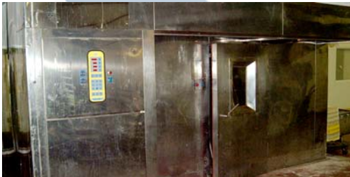
Double D Revorack through door eight rack gas fired oven with CIP system and full program control, also available Double D 2 & 3 rack single door gas ovens.
