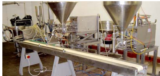
Numerous depositors including Turbo Tools, Unifiller & Baynflax complete with tooling.
