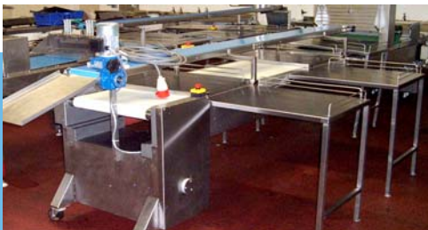
Total Bakery Engineers cake cutting & guillotine lines – fully automatic with work stations to each line.
